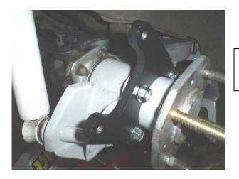
1. Bolt on a brake bracket (not side specific) as shown in the picture. The ears should be toward the back of the car. Torque the bolts to 40 ft-lb.
