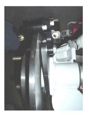
2. Install the disc (rotor) on to the hub. Slip the caliper over the rotor (brake pads installed, and pistons fully retracted). Fasten the caliper to the mounting ears as shown. Use a standard 10mm washer between the caliper and the bracket ears to precisely center the caliper on the rotor. The threaded holes in the mounting bracket are M10X1.5. Torque these bolts to 35 ft-lb using blue Loctite on the threads. Repeat for the opposite side.
