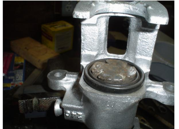
8) Keep turning and pushing the piston in until it is fully inserted. Re-assemble the caliper and install the brake pads.
