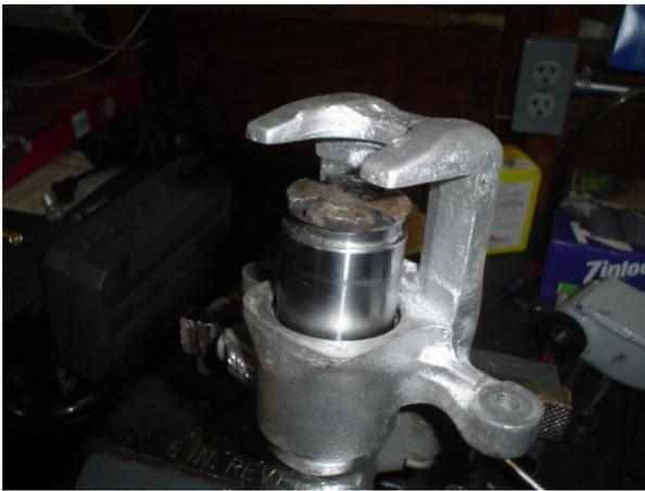
1) Remove the outer dust boot. Pump the E-brake arm until the piston comes out. Inspect the outside of the piston for scratches or pitting, replace if necessary. Pistons from the maxima and 200sx calipers are interchangeable.
