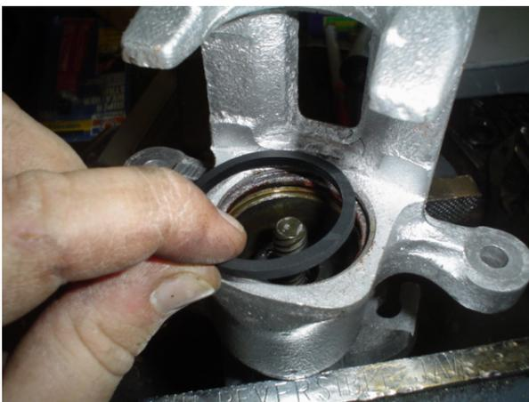
3) Clean out the bore of the caliper and install the new seal from the rebuild kit. Lubricate the sealing surface with a little brake fluid.
