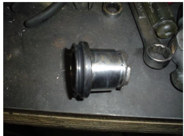
4) Slide the new dust boot on to the cleaned piston. Do not slide all the way on, just get the first lip started.
