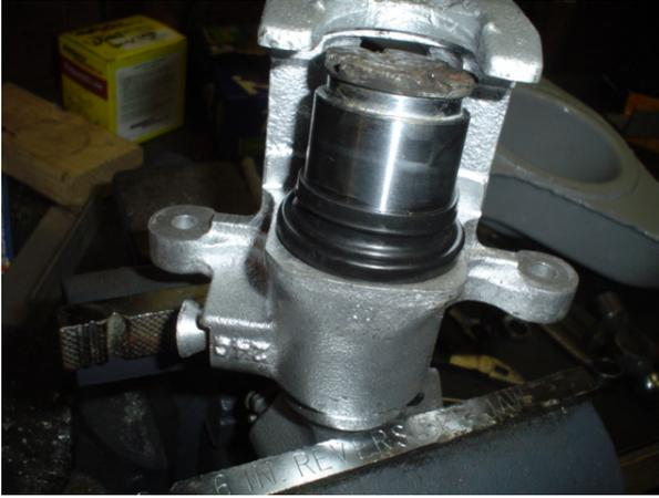
5) Seat the lip of the dust boot into the groove on the inside of the bore of caliper. After the boot is seated in its groove, begin to push the caliper into the bore.
