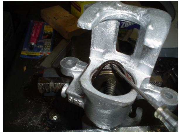
2) Remove the main seal with a pick or similar tool.
