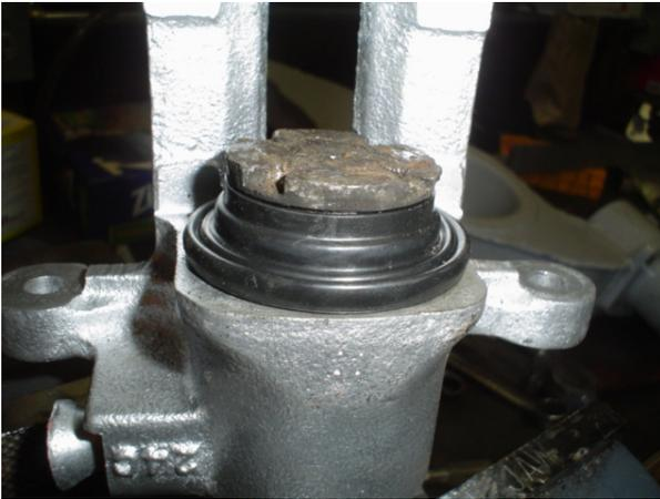
7) When the piston is almost completely in, make sure the rim of the dust boot is seated in the groove on the piston as shown.
