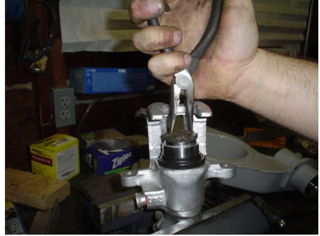
6) Using a set of needle nose pliers, push and turn (clockwise) the piston into the caliper bore. It will begin to thread onto the shaft inside the caliper. As you are pushing, make sure the dust boot is sliding up the caliper.
